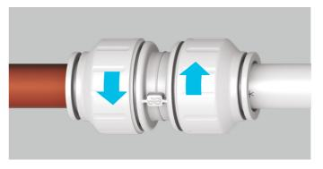
Twist the screwcap until it touches the body flange. This increases the O-Ring seal around the pipe and locks the pipe into position.
