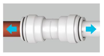
Pull to check connection is secure and test the system. Our recommended test procedure is shown in our Technical Checklist on page 23.
