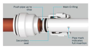
Standard Speedfit connections are made in the same way as Twist  $\&\, Lock.$
