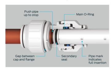
The fitting should be in the 'unlocked' position, this is shown with a small gap between the screwcap and the body flange.
