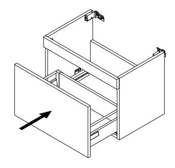
To re-fit the drawer, fully extend the drawer runners and locate drawer box on to runners. Push the drawer box fully home until you here a 'click'. The drawer drawer should now be correctly located onto the runners.
