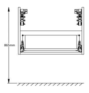
Fix Wall Hanging Plates as shown above. Check the type of wall you are fixing into and use suitable fixings (Not supplied).
