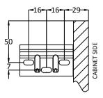
You may need to lengthen the hook's protrusion. To so so, turn screw 'B' anti-clockwise.
