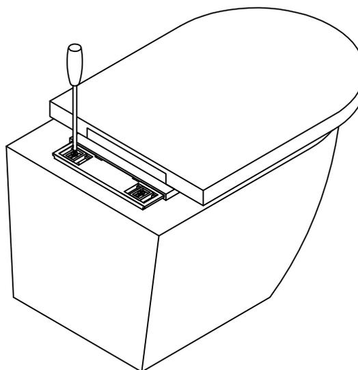
WITH THE FIXING PLATE AND BOLT SETS IN POSITION, SLIDE THE PLATE BACK INTO THE HINGE PLATE 5mm ONLY AS THIS WILL ALLOW ACCESS FOR TIGHTENING THE BOLTS.
